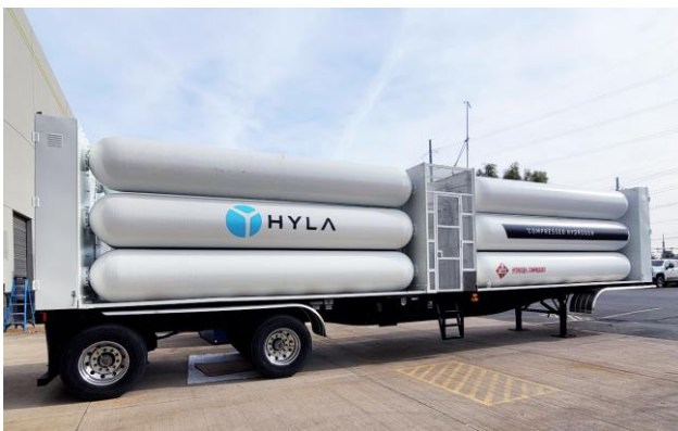
HYL A Hydrogen Tube Trailer
