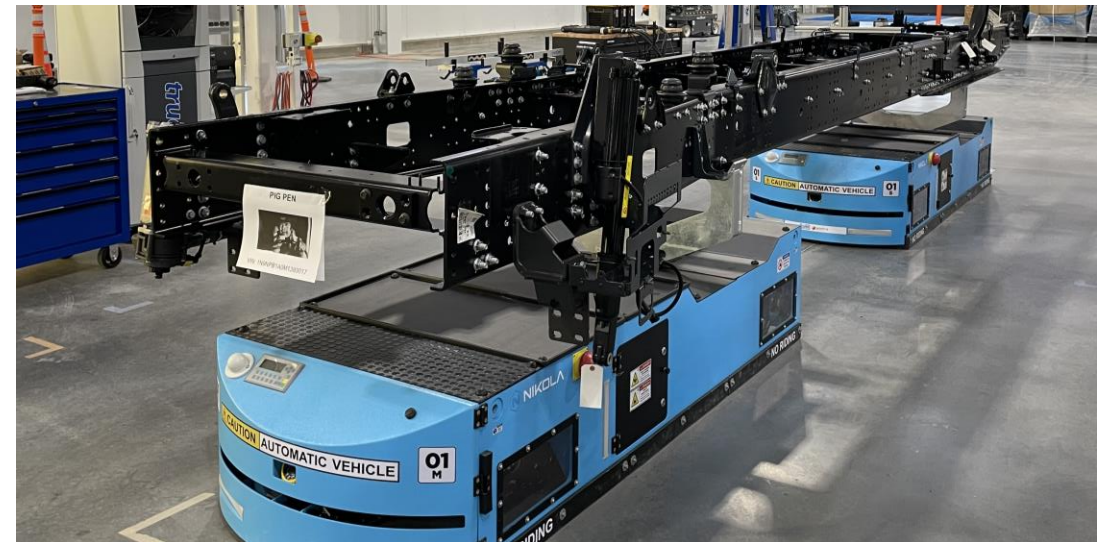
Nikola Tre BEV Frame on AGV in Phase 0.5 of Coolidge
